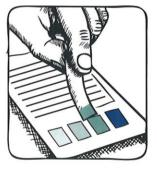
2. At two minutes, compare test pad with the color chart printed on back panel of the foil package. Within 30 seconds choose the closest color match to estimate the alcohol concentration.
